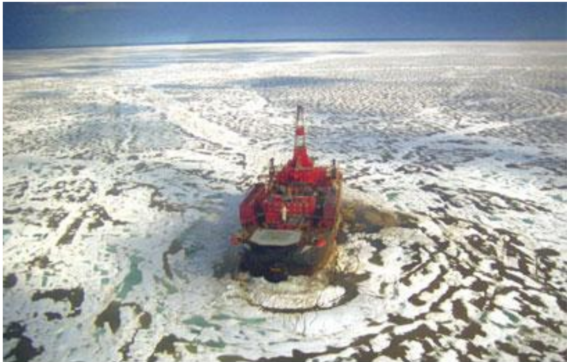
A steel drilling caisson ship in the Beaufort Sea— photo by Challenger Geomatics Ltd.
